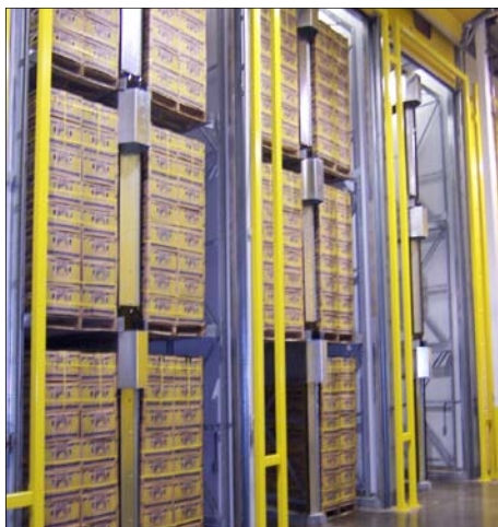
3-Tier 42-Pallet Rooms Single or Dual Temperature Control
